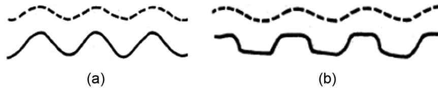
Figure 2. Pre- and post-yield shear stress responses (solid lines) of an ER-based device under oscillatory strain input (dashed line) (Yen and Achorn, 1991): (a) pre-yield region and (b) post-yield region.
